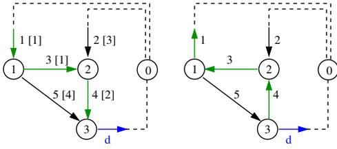
Fig. 3. Super-graph  $\bar{\mathcal{G}}$  and an optimal flow  $\bar{u}$  along the shortest path (left) and residual graph  $\mathcal{R}(\bar{u})$  associated with the optimal flow  $\bar{u}$  (right). Costs are in square brackets.
