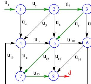
Fig. 1. The network in Example 1. Green arcs identify the shortest (or, more in general, minimum-cost) path from the source node to the sink node.
