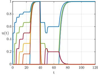
Fig. 4. The time evolution of the arc flows  $u_i$  in the graph in Fig. 1 according to our dynamic algorithm spontaneously leads to the exact minimum cost solution. At time  $T = 40$ , arc 7 undergoes a failure.
