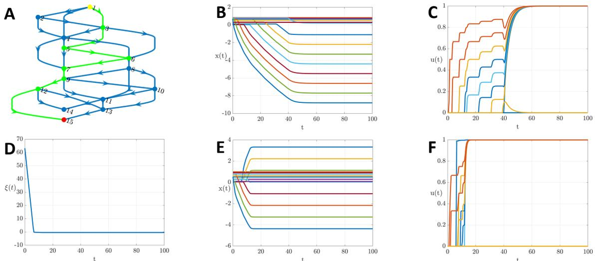
Fig. 5. A: Graph with 15 nodes and 30 arcs. Green arcs identify the shortest (minimum-cost) path from the source node (yellow) to the sink node (red). The arrows on the arcs represent the direction of the flow. Evolution of state (B) and arc flows (C) for system (1) with control strategy (3). Evolution of auxiliary state variable (D), state (E) and arc flows (F) for system (13) with control strategy (14) ( $\eta$  scaled with  $\alpha = 10$ ).
