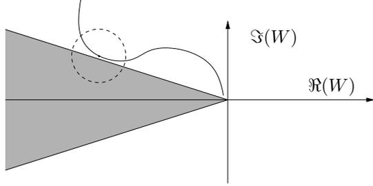
Fig. 3. Nyquist plot of  $W$  not entering the “forbidden” sector  $\mathcal{S}_0$  (shaded). The disk inside the dashed circle represents the uncertainty at a particular frequency.
